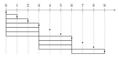
Figure 4: Tumbling time-based window of size 3, bullets indicate query times
