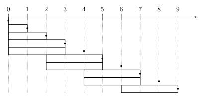
Figure 3: Hopping time-based window of size 3 and hop size 2, bullets indicate query times
