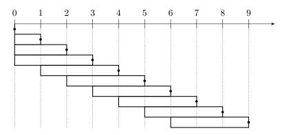
Figure 2: Sliding time-based window of size 3, bullets indicate query times
